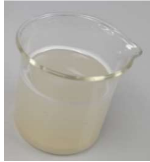
Figure 1: Dispersibility profile in water. [REDACTED] was readily soluble in water and dissolved within 5 minutes.
